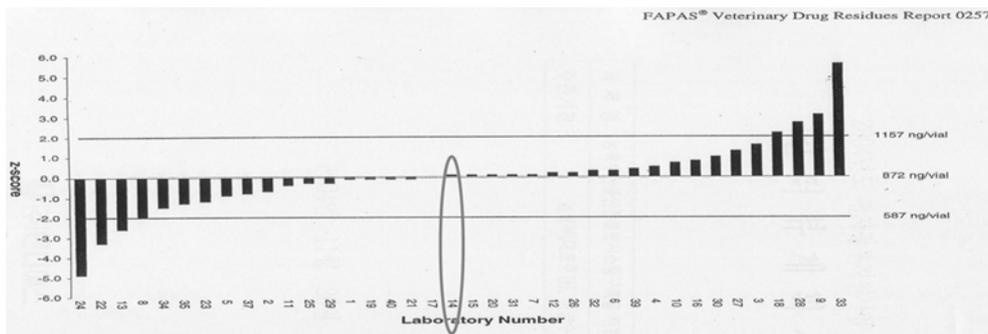
**Fig. 1.** Proficiency test for determination of sulfadimidine.
